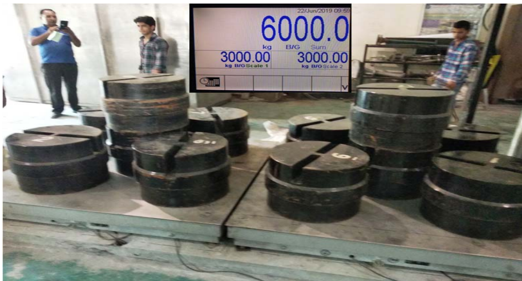
Calibration of 6000 kg Weighing Scale for Performance Evaluation of Primary WFCF
