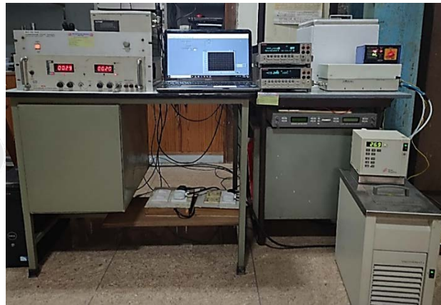
(a) Components Involved in the Development of PID Resistant Solar PV Modules that Sustain the Country Specific Conditions and to Ensure its Long-term Performance as per the Predicted Lifetime, (b) PID Test Facility, which is being Set-up according to the SEMI Test Method (SEMI Draft Document 5889)
