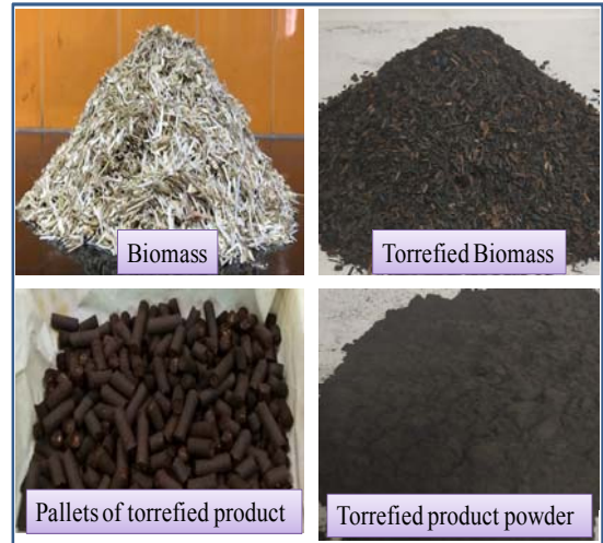
Torrefied Product at Different Stage from Raw Biomass to Torrefied
