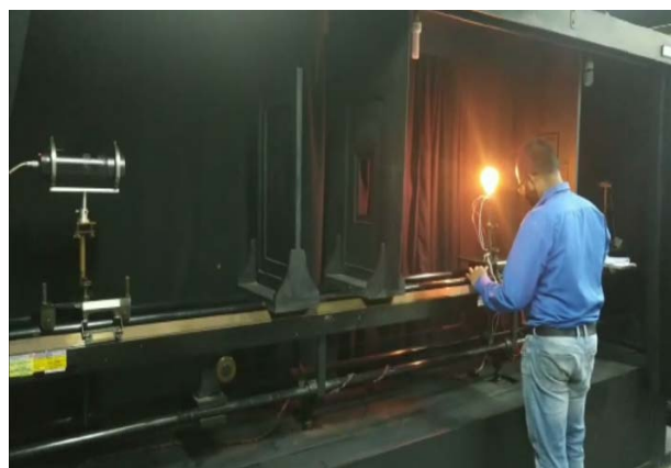
Luminous Intensity and Illuminance Measurement Setup
