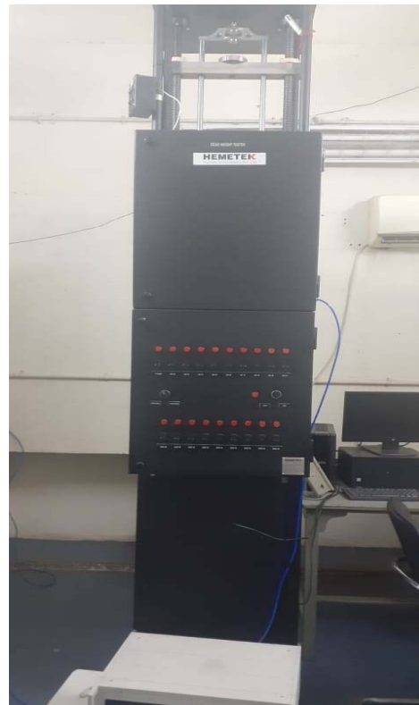
5 kN Dead Weight Force Machine
