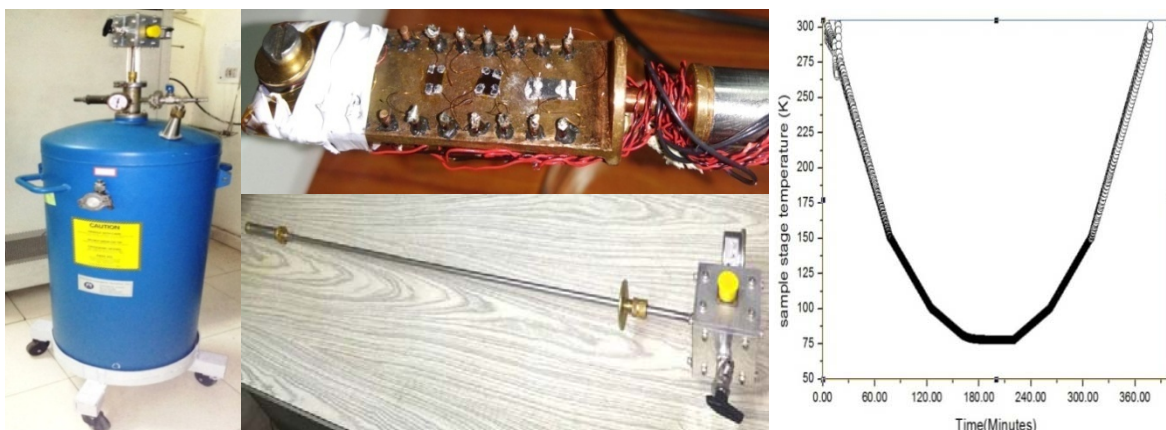
(a) Setup with Probe immersed in Liquid Nitrogen Dewar (b) Lower Part of Probe showing Connections (c) Low Transport Measurement Probe (d) Temperature vs Time Measurement for Increasing as well as Decreasing Temperature
