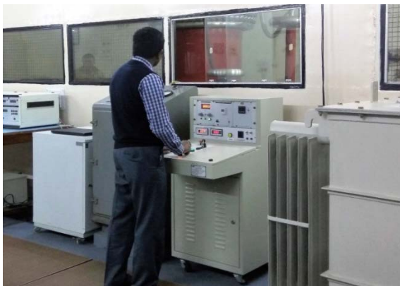
AC High Voltage Setup of 200kV is being Operated for Calibration
