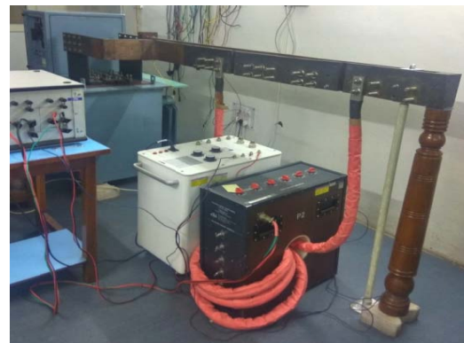
Current Transformer Calibration Set-up
