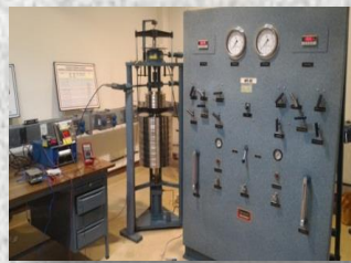
NPL-H1: Primary Pressure Standard for 1GPa
