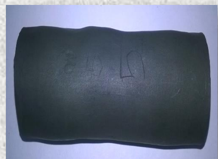
High density graphite after heat treatment at 2350°C
