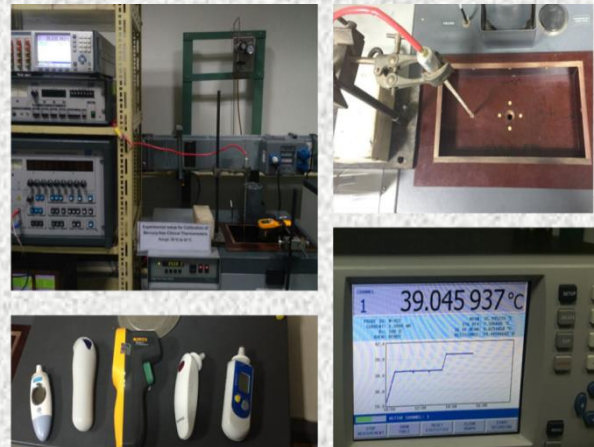
Ear thermometer calibration set up
