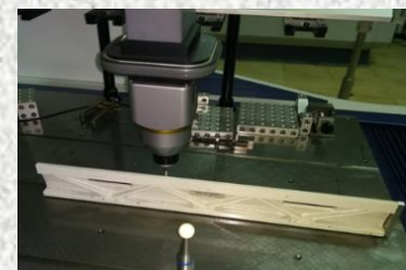
Euramet LK-5 artefact being measured on CMM
